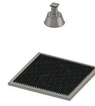
Figure 4. Configuration of the proposed dual-mode reflectarray.
