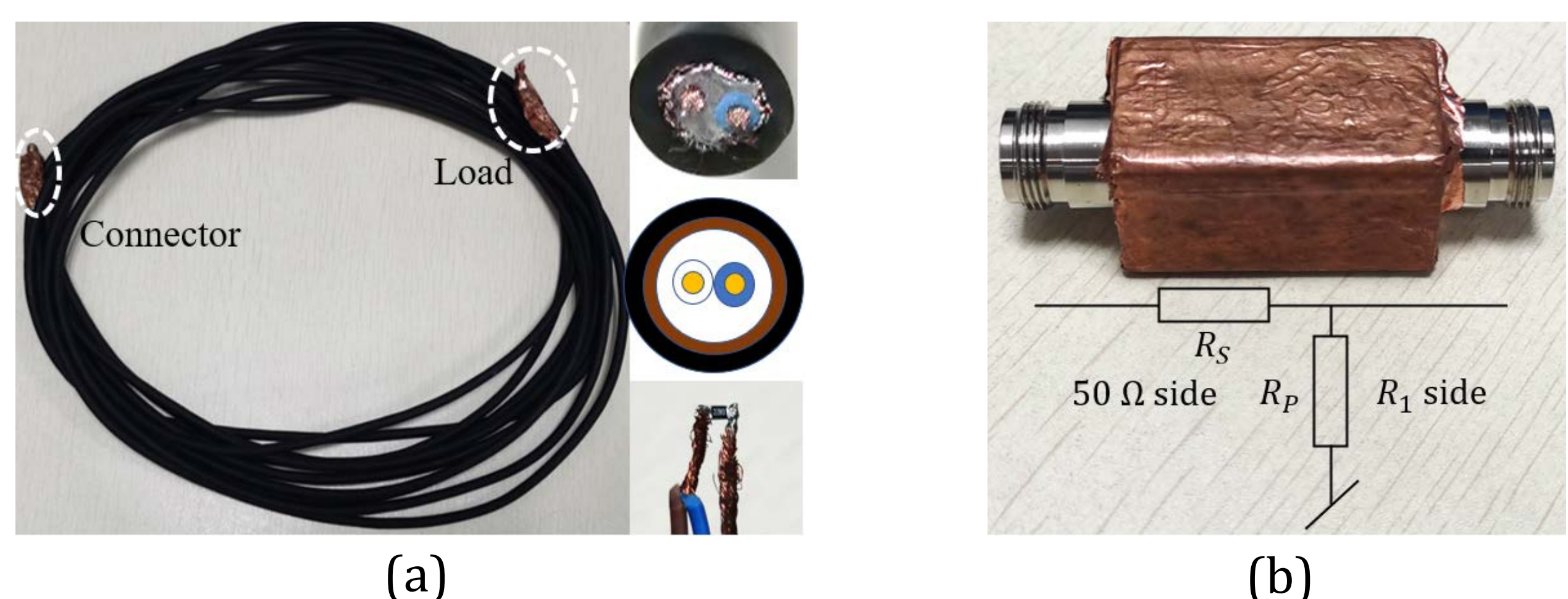
Fig. 3. (a) The paired cable, (b) Impedance adapter.
